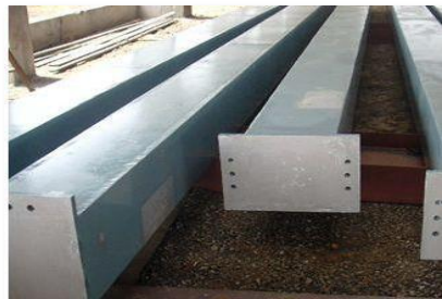
Box columns & girders
